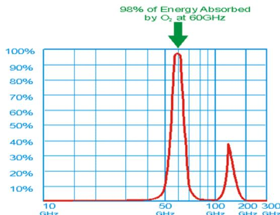
Figure 1: Dry Atmospheric Absorption per Kilometer
